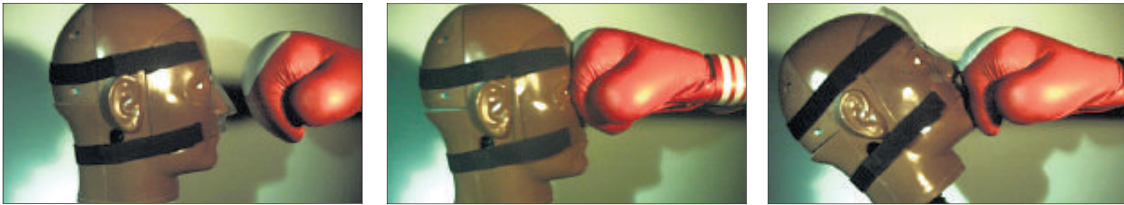
Wayne State University In an injury simulation, a dummy was struck in the bridge of its nose by a boxing glove on a mechanical arm and had a baseball fired at it from about 2 feet. In both tests, the dummy sustained less damage wearing a mask than without. Also, the power of the blow was absorbed by stronger bones in the face.
